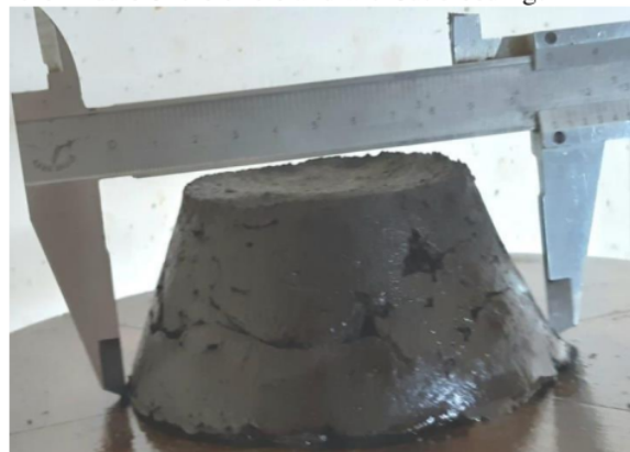
Figure 5. Flow of fresh geopolymer mortar
